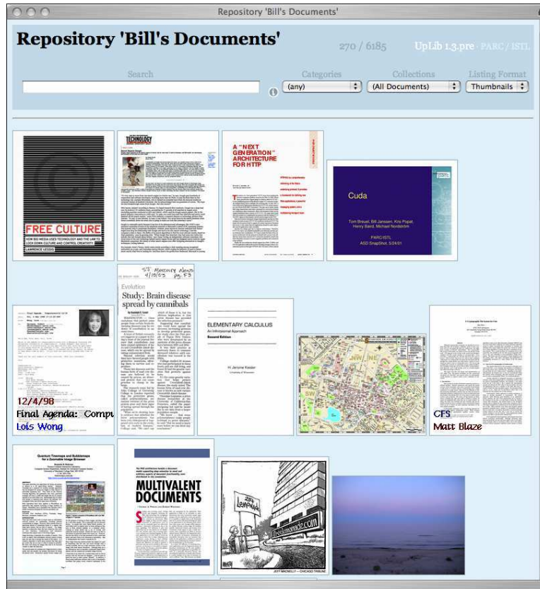
Fig. 1. Document icons in an UpLib overview. These icons are generated using a constant-area algorithm, which allocates the same amount of area to each thumbnail, regardless of orientation. In this interface, clicking on an icon opens that document in a reader program.
